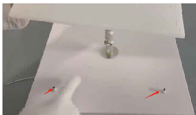
4 small pillars on the chassis snap the lampshade
