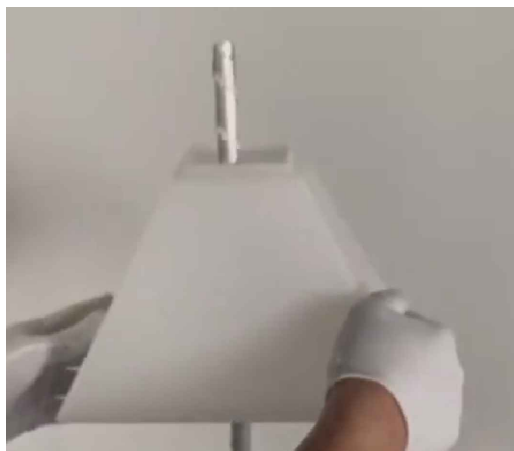
The lampshade is put into the light pole
