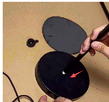
The A rod is passed into the round hole of the chassis and tightened with a nut
