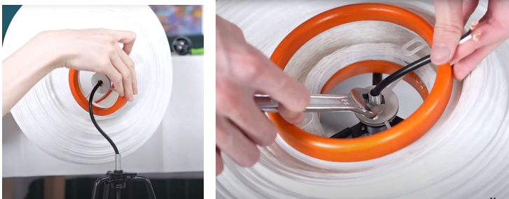
2. The power cord passes through the lampshade and is fixed
