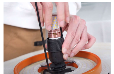
3. Connect the lamp head wires and install the light bulb
